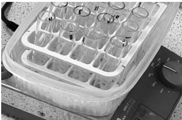
Figure 1. Arrangement of ice-water bath over a magnetic stirrer for dissolution/hydration of \beta -glucan in KOH.
