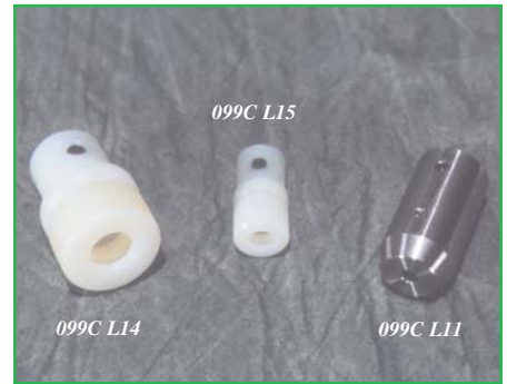
L14 and L15 fit Glas-Col motors or any motor with a 5/16" shaft. L11 chuck requires c.c.w. motor rotation.
